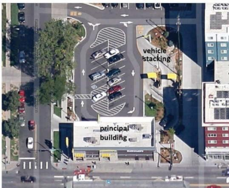
Figure 1129.46 (6). Recommended Drive-Through Facility Layout.
