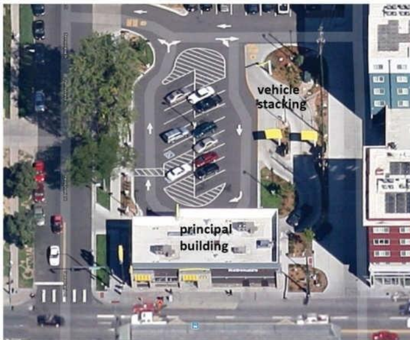
Figure 2332 (6) Recommended Drive-Thru Facility Layout
